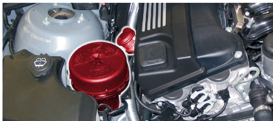
Secondary air valve and secondary air pump in BMW E46 (highlighted)
