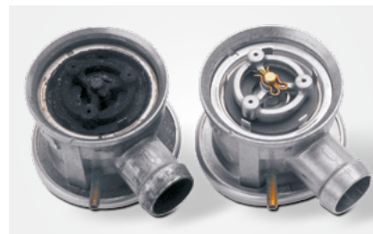
Open secondary air valve Left: Damage caused by exhaust gas condensate Right: New condition
