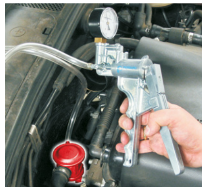
Checking a secondary air valve with a vacuum hand pump
