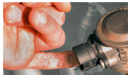
Finger test at secondary air valve in BMW 520i (highlighted) If deposits are found on this end, the non-return valve is leaking and must be replaced.
