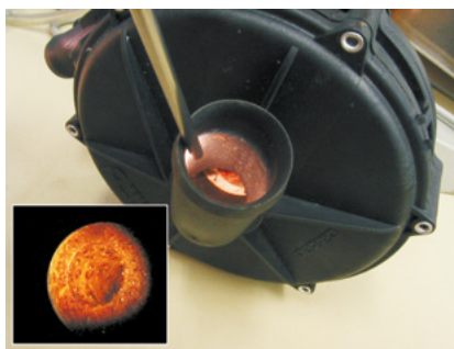
View of the corroded inlet of a secondary-air pump
